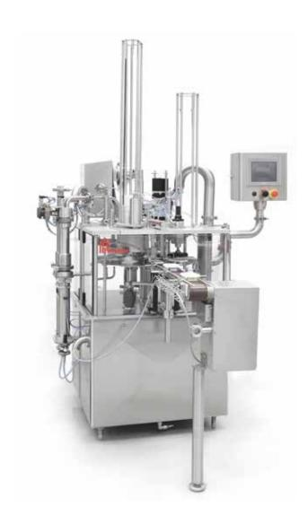
Rotary filling and sealing machine
